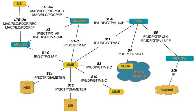
Fig. 1. LTE Architecture and Protocols
